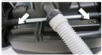
3. Turn the machine upright and remove the wheel caps. Use a small flat head screwdriver to pry off caps.
