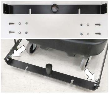
6. Connect the squeegee pedal to the lift arms and lower support bracket using hardware as shown.
