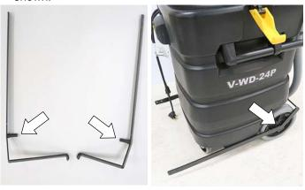
Connect the squeegee mount plate to the lift arms using hardware as shown.
