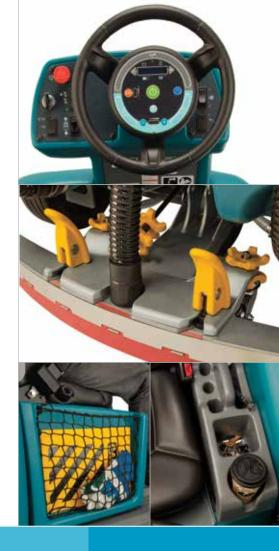
Effectively clean along edges with the scrubbing side brush that expands cleaning path for maintenance cleaning productivity. Bring high performance spill recovery to hard-toreach areas with the in-line telescoping vac wand. Reduce repair costs and protect the rear squeegee when backing up with the rear squeegee protection kit. Protect operators from falling objects with the overhead guard and protect the T16 from contact damage with the severe environment front bumper.
